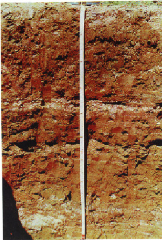
Plate 5.b. Soil Profile. Sandy Clay Loam in A, B and C. Light brownish gray in A and light gray in B and C horizon.
