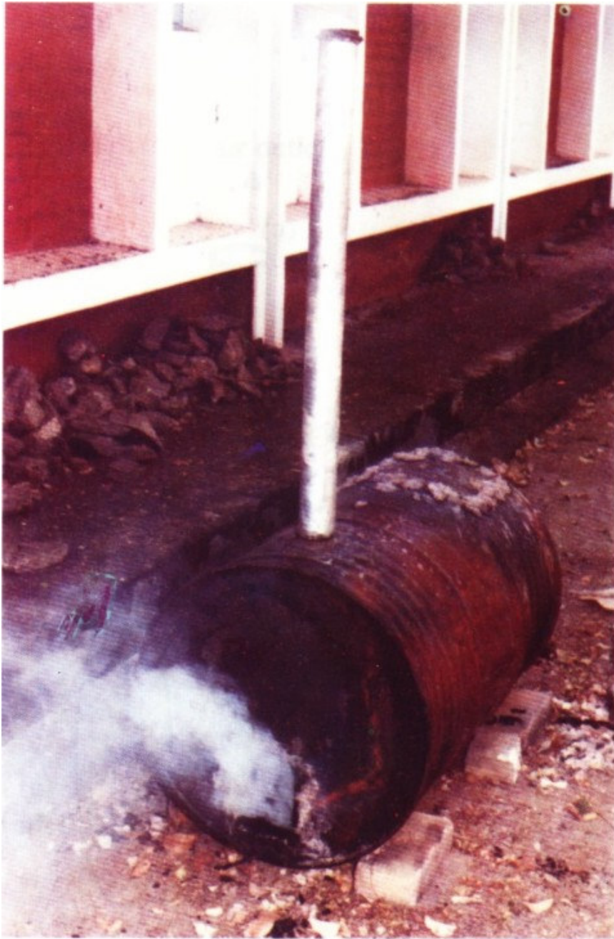
Fig (3) Production of activated carbon by using old oil drum.
