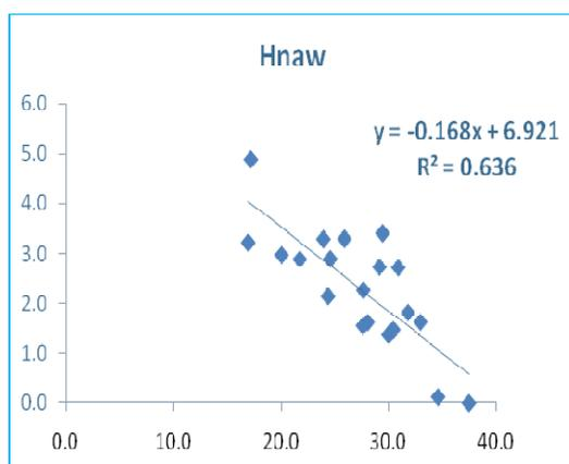
Fig: (4.6) The relationship between WPG and weight loss (%)for acetylated Hnaw samples
