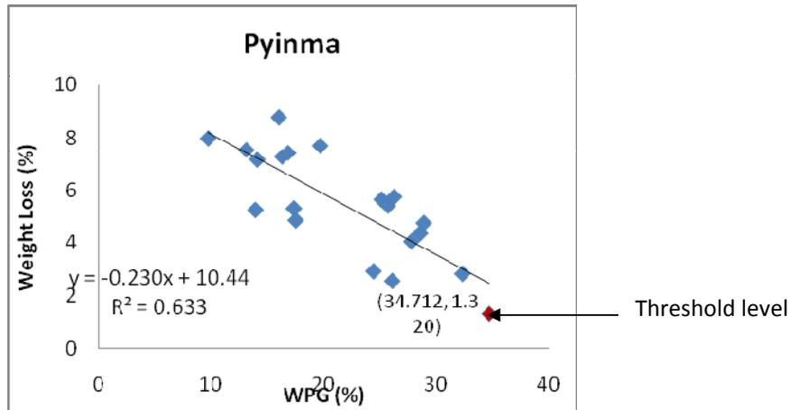
Fig: (4.14) The relationship between WPG and weight loss (%) for acetylated Pyinma samples
