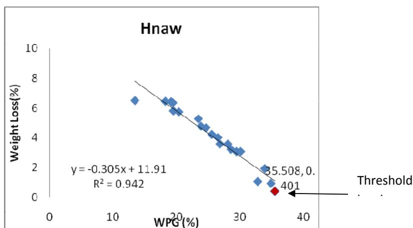
Fig: (4.12) The relationship between WPG and weight loss (%) for acetylated Hnaw samples
