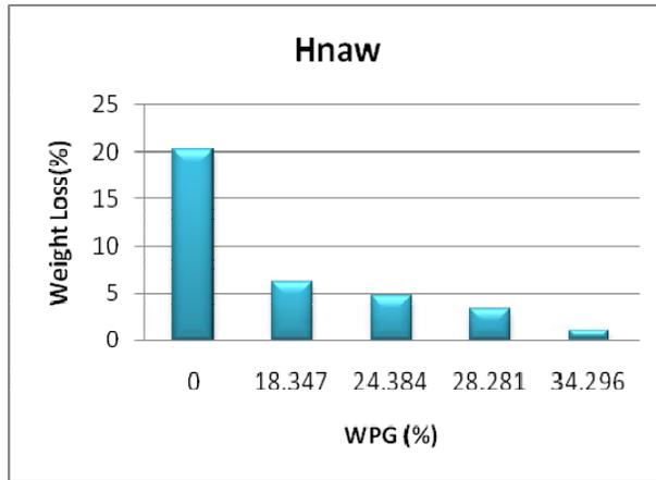
Fig (4.9) Weight loss (%) of un-acetylated and acetylated Hnaw samples after 16 weeks exposure in soil bed
