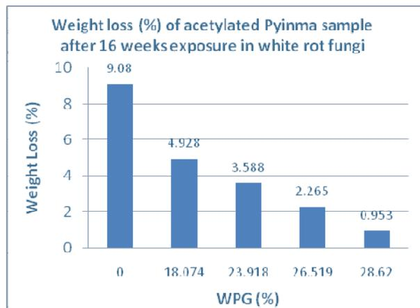
Fig (4.5) The weight loss (%) of Pynma samples after 16 weeks exposure
