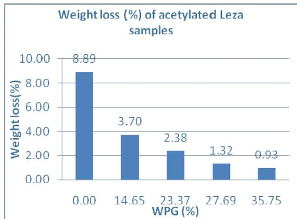
Fig (4.4) The weight loss (%) of Leza samples after 16 weeks exposure
