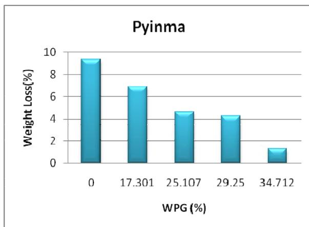
Fig 4.11 Weight loss (%) of un-acetylated and acetylated Pyinma samples after 16 weeks exposure in soil bed
