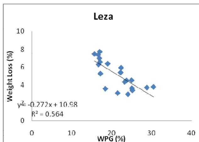
Fig: (4.13) The relationship between WPG and weight loss (%) for acetylated Leza samples
