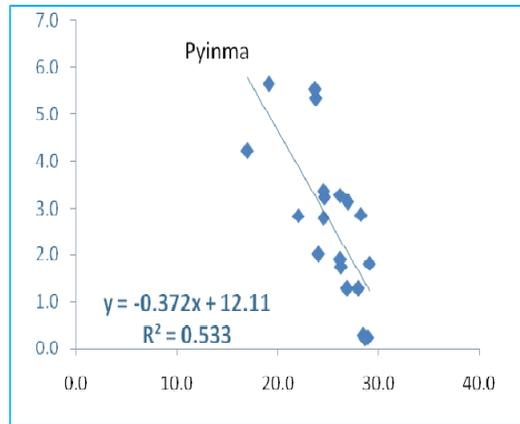
Fig: (4.8) The relationship between WPG and weight loss (%) for acetylated Pyinma samples
