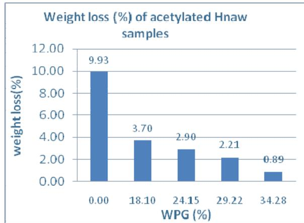
Fig (4.3) The weight loss (%) of Hnaw samples after 16 weeks exposure
