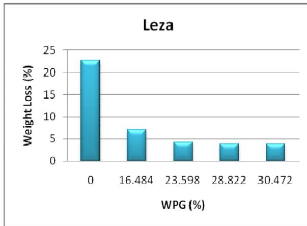
Fig 4.10 Weight loss (%) of un-acetylated and acetylated Leza samples after 16 weeks exposure in soil bed
